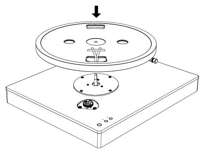
2. Install the belt drive. Make sure that the belt is installed properly around the motor.
