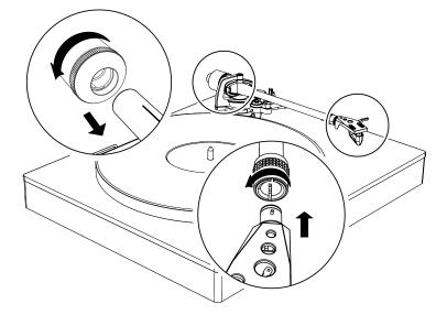
3. Release tonearm from rest and remove the stylus guard.
